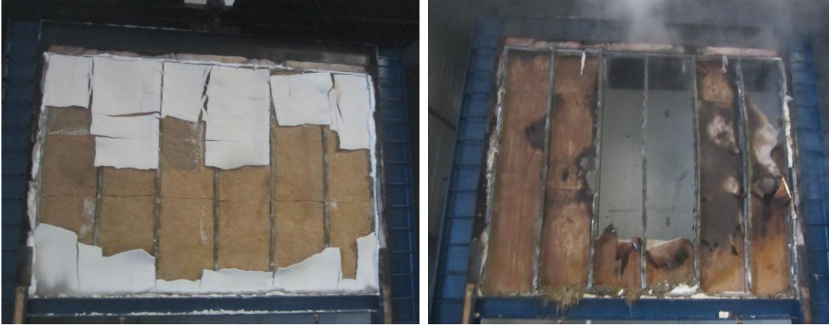
3. The exposed face after the fire test and immediately after the hose stream test.
