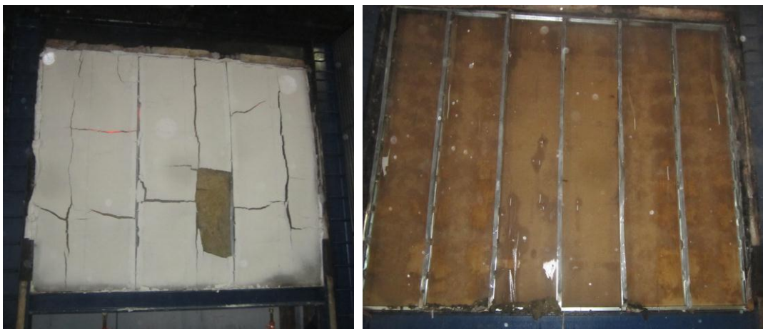
2. The duplicate test sample after the fire and hose stream test.
